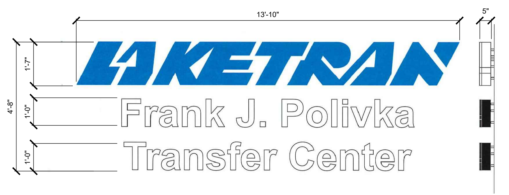
FACE & HALO LIT CHANNEL LETTERS SCALE: 1/2" = 1'-0"
