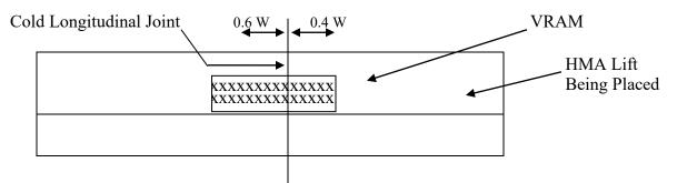
Apply VRAM at the width and application rate required according to the following table:
